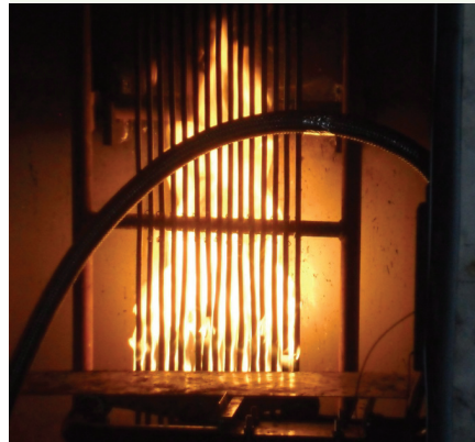
Reaction to fire test according to EN 50399 standard
