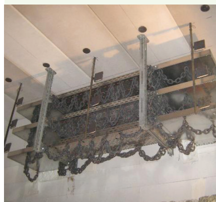
Fire resistance test according to prEN 50577 standard
