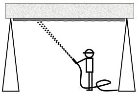
Figure 2.2.1: Overhead spraying of spray mortar
