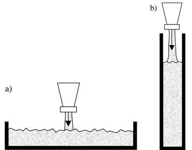
Figure 2.1.1: Specimens cast in the correct position; a) wall or ceiling; b) wall
