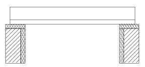
C. Cross section I-I: slab with sprayed insulation material
