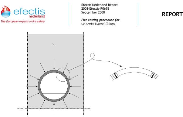
Figure 2.1.2: Principle of representing compressive ring forces by prestressing
