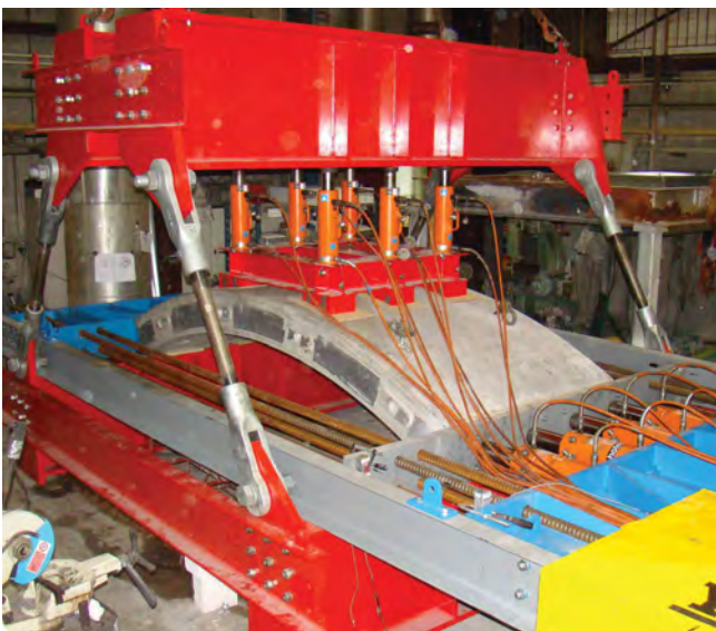
Loading frame used for fire testing of bored tunnel linings
