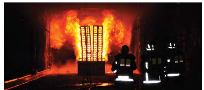
Full scale tunnel fire test with activated deluge fire suppression system
