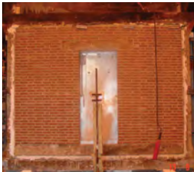
Fire resistance test on tunnel door in front of the vertical furnace at Efectis Nederland
