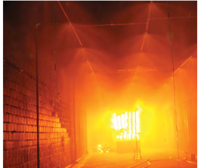
Full scale fire test in progress in the TST test facility in Spain
