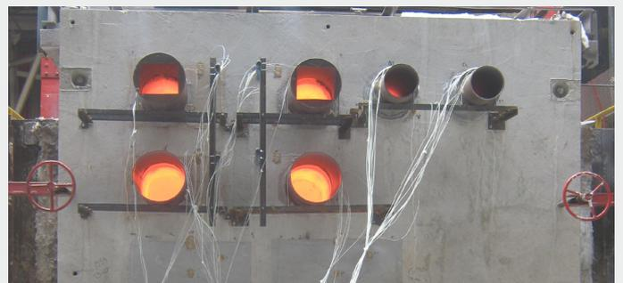
Fire test on penetration seals
