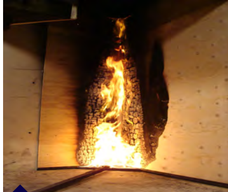
SBI test according to EN 13823
