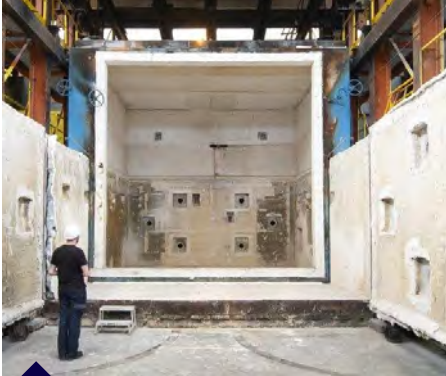
G furnace 24 MW 1000 tonnes 8x6x5 m (LxWxH)
