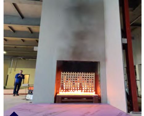
Test according to BS 8414 standard
