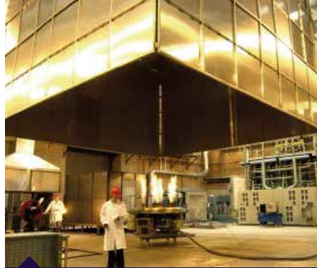
Large calorimeter 10 MW 9x9x9 m
