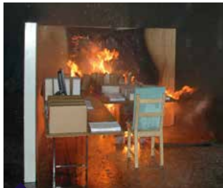
OH1 test for watermist systems
