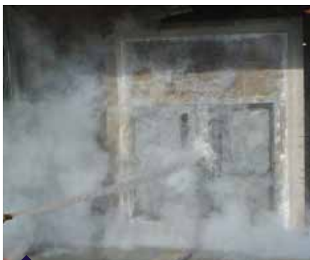
Hose stream test (2 bar) applied just after the fire test
