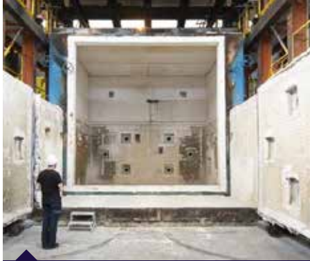
G furnace 24 MW 1000 tonnes 8x6x5 m (LxWxH)
