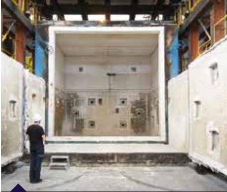
G furnace 24 MW 1000 tonnes 8x6x5 m (LxWxH)
