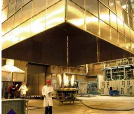
Large calorimeter 10 MW 9x9x9 m
