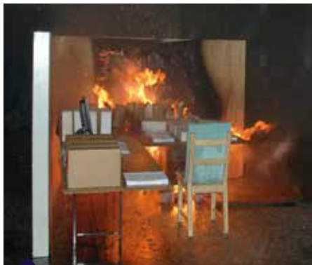
OH1 test for watermist systems
