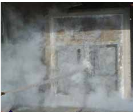
Hose stream test (2 bar) applied just after the fire test
