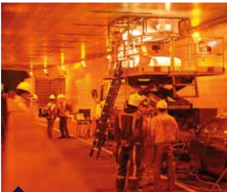
Fire test on an existing tunnel wall using our MobiFire®
