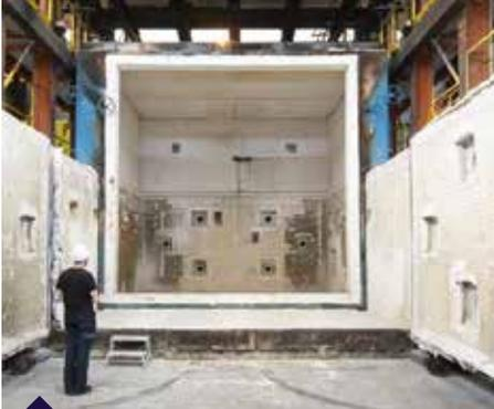
Four G 24 MW 1000 tonnes 8x6x5 m (LxlxH)
