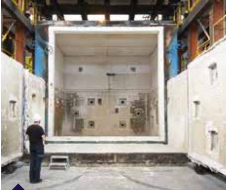
G Öfen 24 MW 1000 Tonnen 8x6x5 m (LxBxH)
