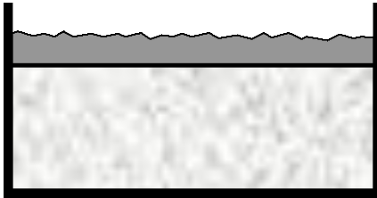
Figure 2.3.2: Concrete sample in its formwork, with spray mortar applied to the top surface
