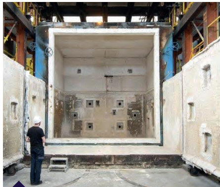
Four G 24 MW 1000 tonnes 8x6x5 m (LxlxH)
