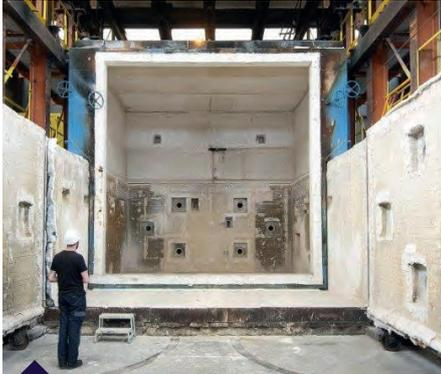
Four G 24 MW 1000 tonnes 8x6x5 m (LxlxH)
