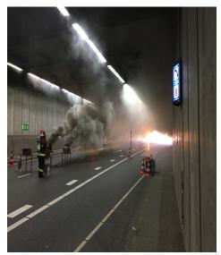
Tunnel safety actors must be properly prepared to deal with any event occurring in the tunnels. Regular safety exercises or drills are a good way to maintain their ability to respond effectively. The generation of smoke and heat brings a high degree of realism allowing participants to be placed in conditions close to what they might encounter in the field.
