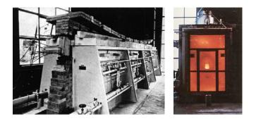
strongly supported by the ministry of Reconstruction. The business association "De Betonvereniging" wished to continue the research projects on pretensioned concrete and the behaviour in case of fire. Despite the ambition of a furnace up to 12 meters long, a testing furnace for a pretensioned loaded concrete beam with a length of 'only' 8 meters was designed and built in 1954.
