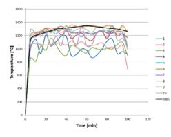
A total of 10 thermocouples were used to measure the temperatures in the tunnel during the fire test. Out of the 10 thermocouples, 9 were placed at a distance of 0.1 m from the concrete slabs at the ceiling, whereas 1 thermocouple (number 3) was placed at half of the height of the tunnel, hence we will observe the 9 thermocouples.
