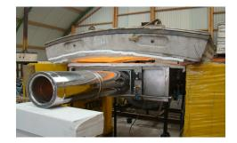
The knowledge obtained regarding the thermal insulation requirements enabled Efectis to assess the performance of several passive fire protection systems in case of a tunnel fire. Based on the assessment of the passive fire protection systems the client was able to select the best solution.
