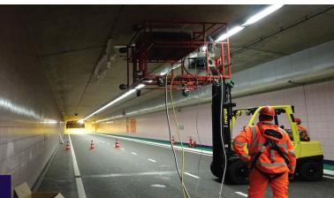
Efectis is the first company in the world that is able to perform realistic fire resistance testing on-site using a mobile furnace. The brand name of the mobile furnace concept is the MobiFire®, which stands for Mobile Fire Resistance.
