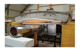
The knowledge obtained regarding the thermal insulation requirements enabled Efectis to assess the performance of several passive fire protection systems in case of a tunnel fire. Based on the assessment of the passive fire protection systems the client was able to select the best solution.
