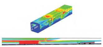
CFD simulations of temperature development and fire behaviour of rolling stock during a fire in the Channel Tunnel
