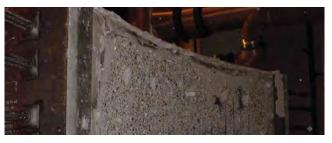
Exposed side of a tunnel segment after a fire resistance test. Spalling of concrete uncovered the reinforcement inside the concrete.
