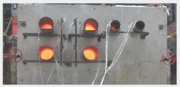
Fire test on penetration seals
