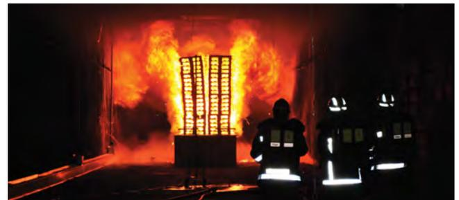
Full scale tunnel fire test with activated deluge fire suppression system
