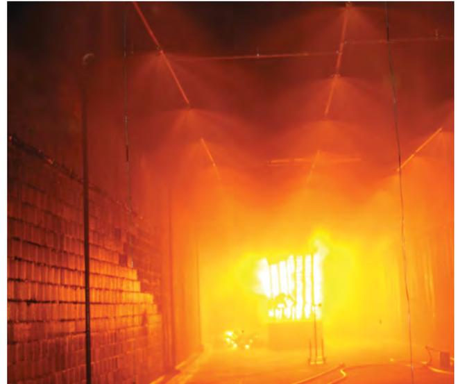
*Full scale fire test in progress in the TST test facility in Spain*
