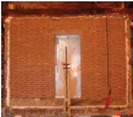
*Fire resistance test on tunnel door in front of the vertical furnace at Efectis Nederland*
