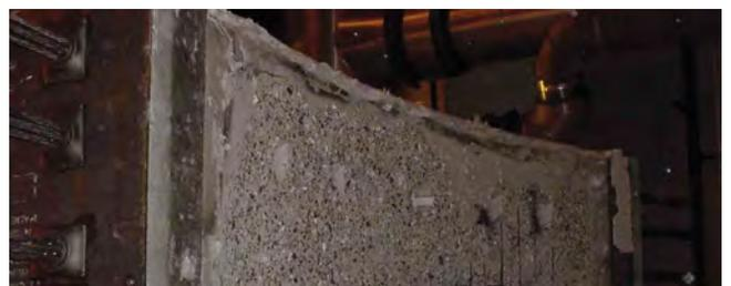
*Exposed side of a tunnel segment after a fire resistance test. Spalling of concrete uncovered the reinforcement inside the concrete.*
